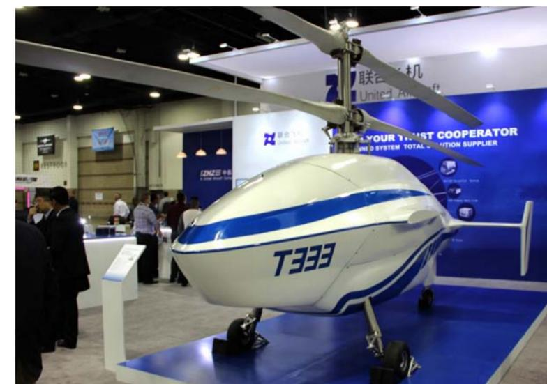
Above right: The Beijing-based drone manufacturer Zonghangzhi Technology produces this large-scale T333 coaxial dual-rotor UAV. It is seen, here, at the 2018 AUVSI Xponential conference in Denver, Colorado.
