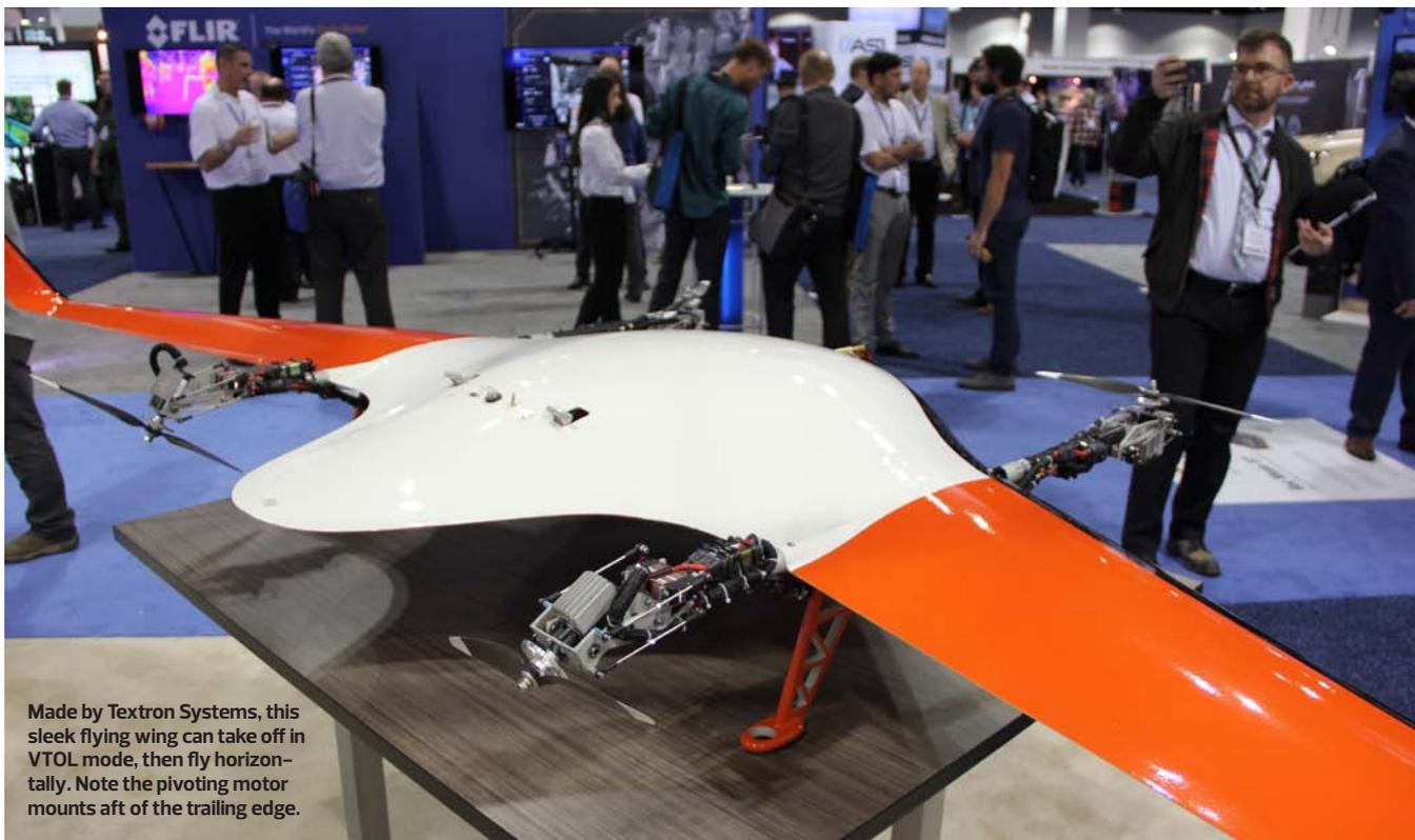
Made by Textron Systems, this sleek flying wing can take off in VTOL mode, then fly horizontally. Note the pivoting motor mounts aft of the trailing edge.
