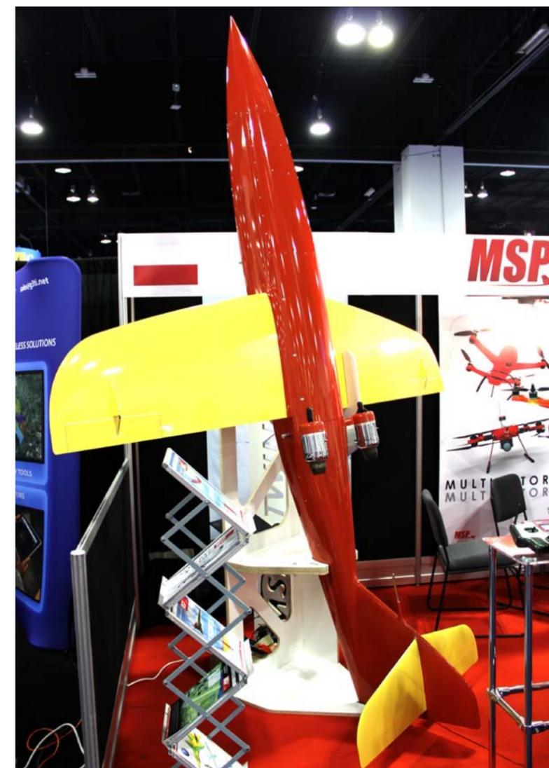
Right: MSP produces diverse robotic aerial vehicles. Not all need to be brainy. In Target mode, this sleek, turbine-powered machine will only require military-grade radio control.
