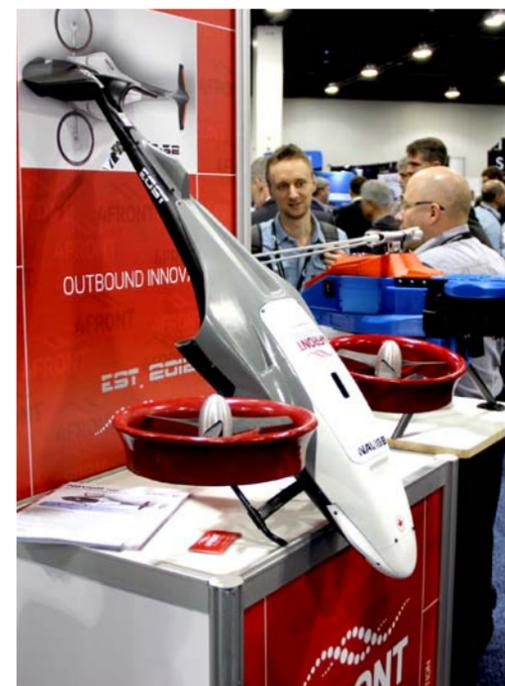
Above: 4Front Robotics, based in Calgary, Alberta, produces this twin multirotor. It is used in search-and-rescue efforts and infrastructure surveys.
